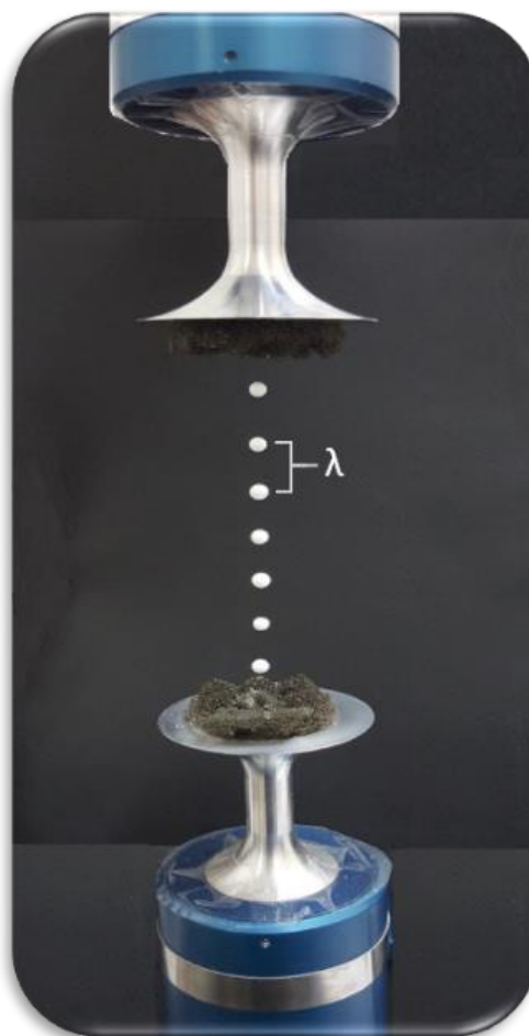
Figure 2.8. Standing waves in an acoustic levitator which furnish stable equilibrium locations for levitated particles.
