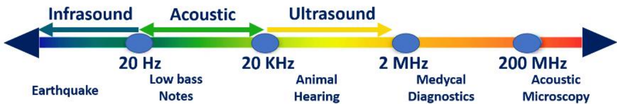
Figure 2.5. Field of audibility (upward). Sound range diagram (below), from infrasounds to ultrasounds. Acoustic waves perceived by human ear span, with a different weight, from 20 Hz to 20 KHz.
