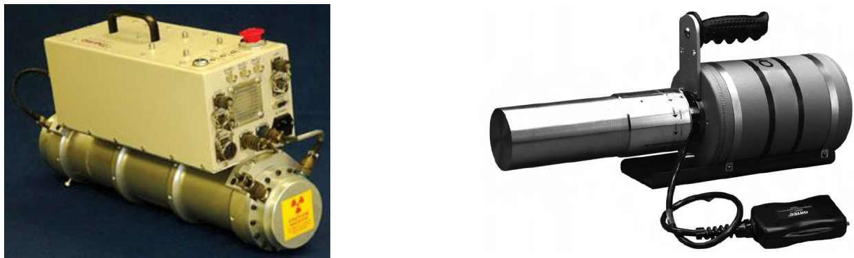
Figure 2: MP320 neutron generator of Thermo Scientific in conjunction with a PINS-GMX Ortec solid-state photon detector.
