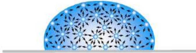
Fig. 3.2 Surface tension is caused by the unbalanced forces of liquid molecules at the surface.
