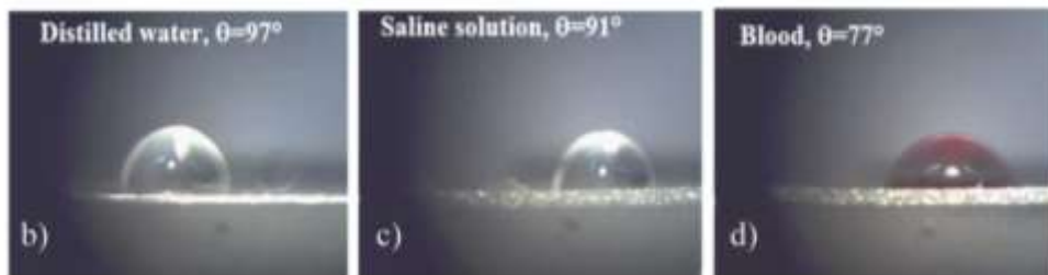
Fig. 3.3- Surface roughness as a function of the nature of the substrate submitted to submicrometric polishing procedure a) and a typical roughness profile in polished copper as inset picture. The vertical bar represents the experimental errors of the order of 6%. Contact angle of distilled water, physiologic saline solution and human blood, using a liquid in which 0.37mg Au NPs/ml were enclosed and deposited on a polished polyethylene surface b).
