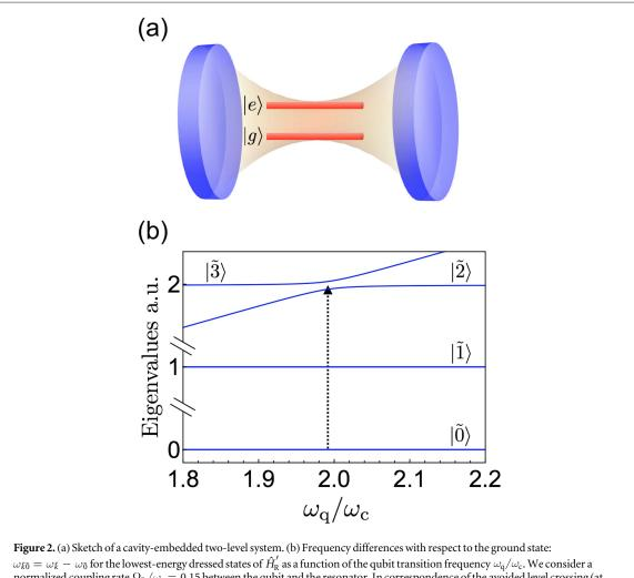
$\omega_{k0} = \omega_k - \omega_0$  for the lowest-energy dressed states of  $H_R$  as a function of the qubit transition frequency  $\omega_q/\omega_c$ . We consider a normalized coupling rate  $\Omega_R/\omega_c = 0.15$  between the qubit and the resonator. In correspondence of the avoided level crossing (at  $\omega_q \approx 2\omega_c$ ) a Gaussian pulse is sent with central frequency in the middle of the two split transition energies (black arrow).
