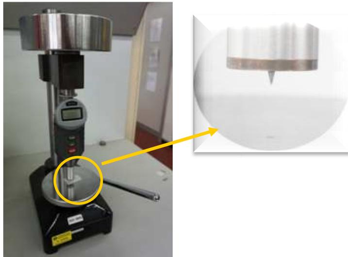
Figura 2.10 - Durometro Shore D PCE-HT 210.
