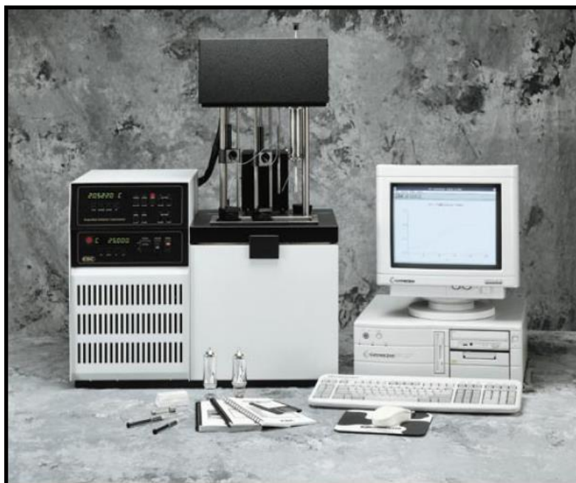
Figure 1.1. CSC isoperibolic calorimeter
