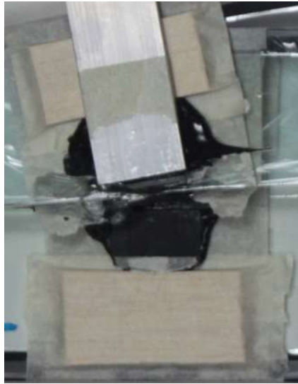
Figure 2.9 Failure modes of glass-GFRP/aluminum double lap joints: adhesive failure.
