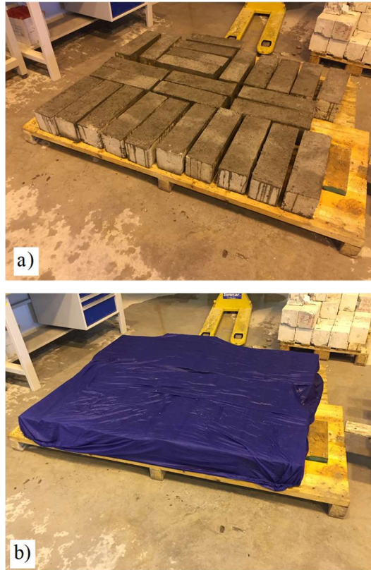
Figure 5.2 Curing process of the specimens: a) after demolding; b) wrapping of specimens to prevent evaporation of water during the 28 days curing time
