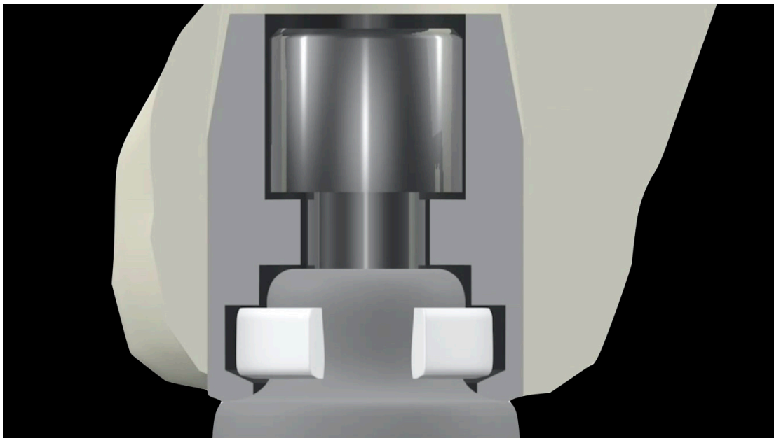
Figure A14. Seeger seal inside OT equator (Rhein83, Bologna, Italy).
