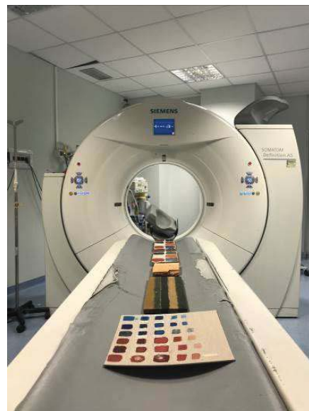
Fig. 1 – Wooden tablets, painted with the most used ancient pigments are placed on the CT scanner bed for the MSCT scanning
