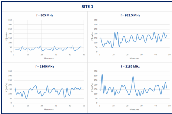
Figure 4. Electromagnetic field values at different frequencies (f = 805 MHz, 932.5 MHz, 1860 MHz and 2135 MHz) for Site 1. Base station distance of 7 meters
