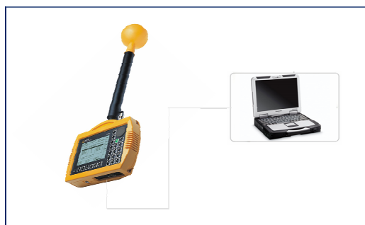
Figure 2. NARDA SRM-3000 data acquisition system
