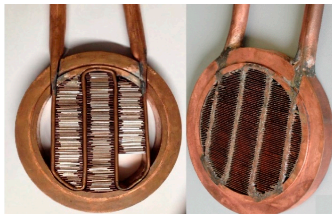
Figure 4. The finned-tube heat exchanger during the fabrication phase (on the left) and after the fin brazing.
