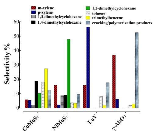
Figure 4. Product distribution in the o-xylene HDT process recorded at 24 h of t.o.s.
