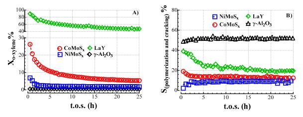
**Figure 3.** Catalytic results: (**A**) conversion of o-xylene and (**B**) selectivity to polymerization and cracking products.
