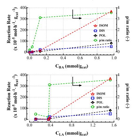
**Figure 5.** Correlation between catalytic data and the concentration of Brønsted and Lewis acid sites determined by FTIR measurements.
