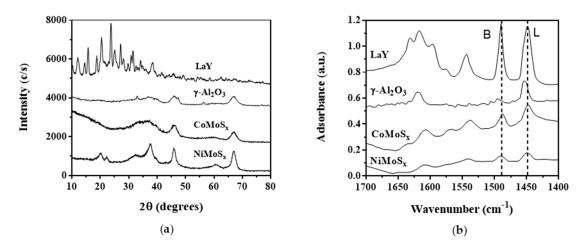
**Figure 1.** (a) X-ray diffraction patterns and (b) Fourier-transform infrared (FTIR) spectra of adsorbed pyridine of catalysts.
