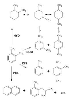
Figure 2. Reaction network of o-xylene hydrotreating (HDT).
