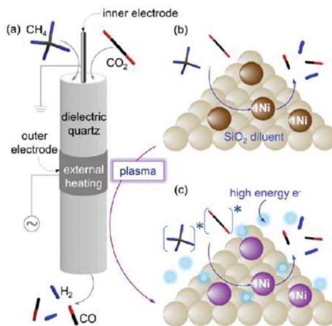
Figure 16. Schematic representation of DRM (a) reactor set-up, (b) thermal catalysis, (c) DBD plasma-assisted catalysis. Adapted from [129] with permission of The Royal Society of Chemistry.
