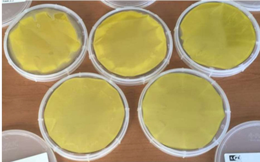
Figure 29 Free-standing 4 inch wafers of 3C-SiC. The growth was performed in a horizontal hot-wall chemical vapour deposition (CVD) reactor supplied by LPE.
