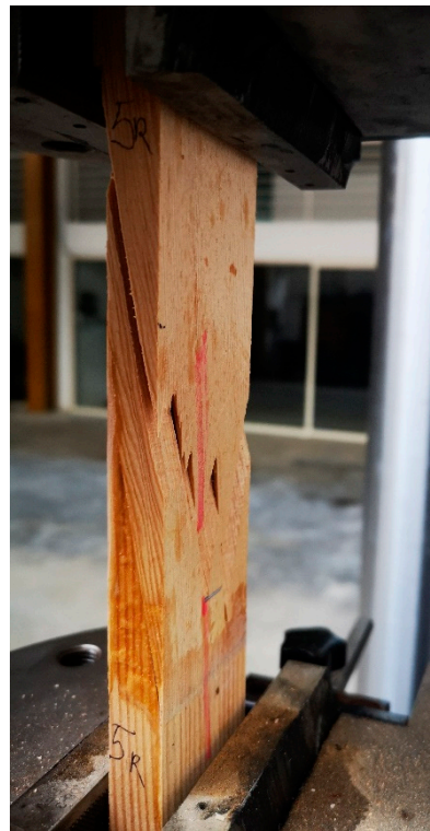
Figure 4. Scarf-joint after rupture.
