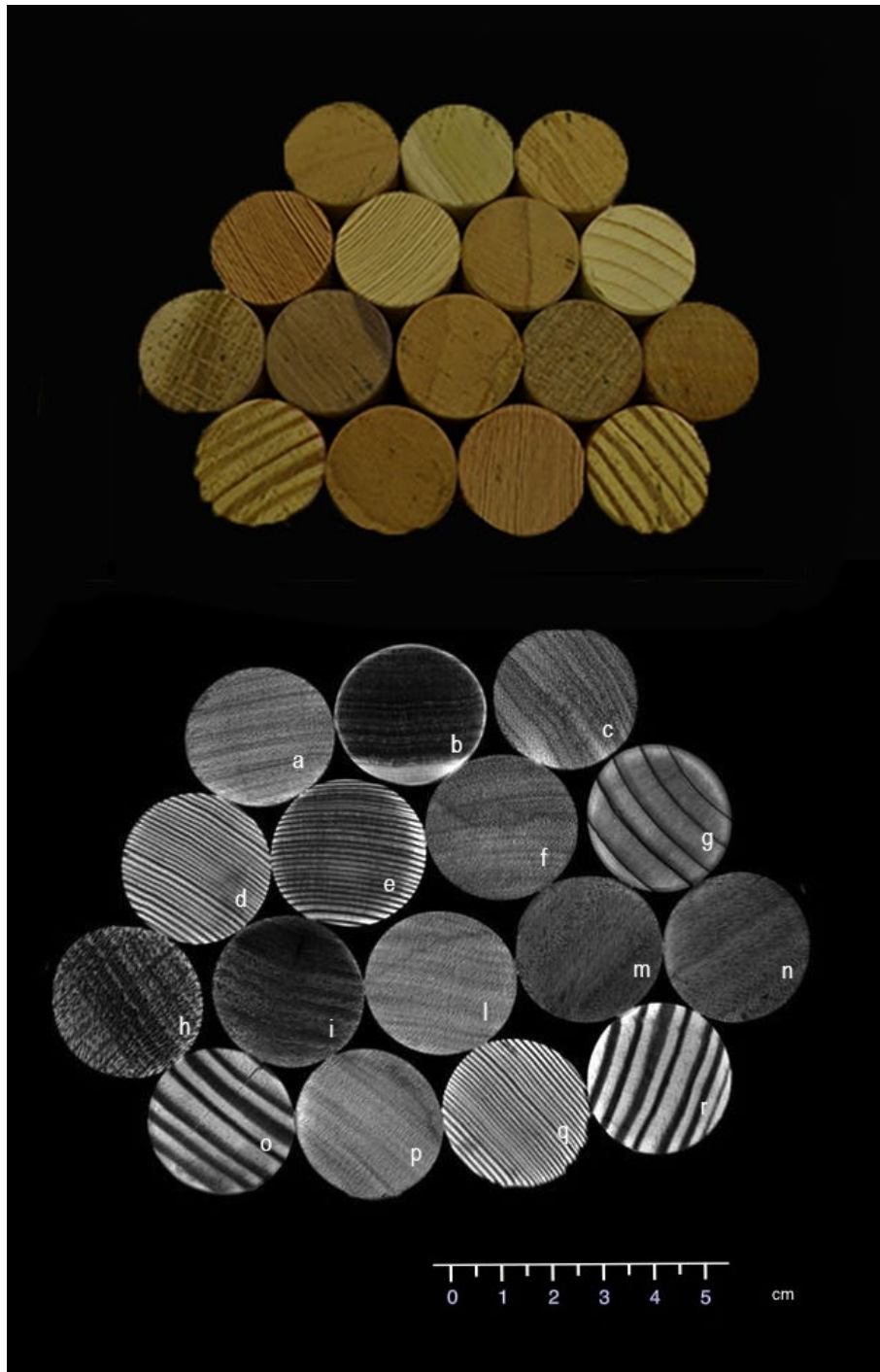
Figure 10a - Photograph image of the soaked contemporary wood samples before scanning NMR. 10b Image position of the samples within the clinical scanner with corresponding letter in the table of right (Longo et al. 2020, in preparation for Wood Science and Technology).
