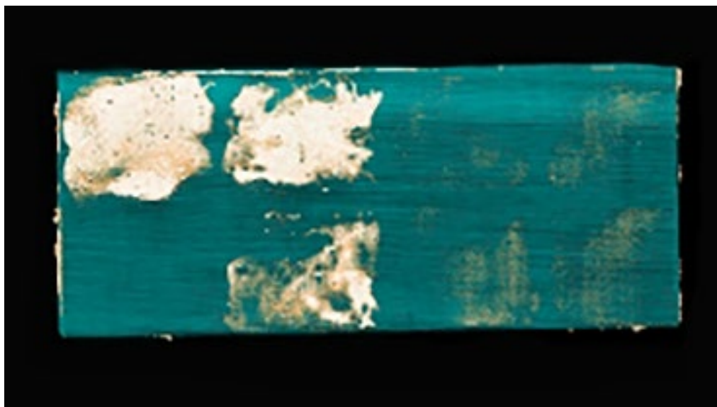
Figure 8 – Bones and skin VRT filter applied on the wooden painted sample. White areas correspond to pigments based on lead and mercury and blue colour zones to wood (Longo et al. 2020, submitted to Studies in Conservation).
