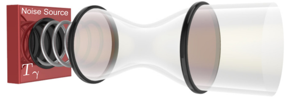
FIG. 1. Schematic of a generic optomechanical system. One of the mirrors of the optical cavity is coupled to a noise source with effective temperature T_\gamma and can vibrate at frequency \omega_m . This system can generate Casimir photon pairs.
