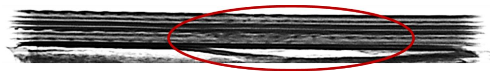
Figure 15. A particular of radiographic inspection for Type V specimen subjected to an impact of 35 J. Skin damage is highlighted by the red circle.
