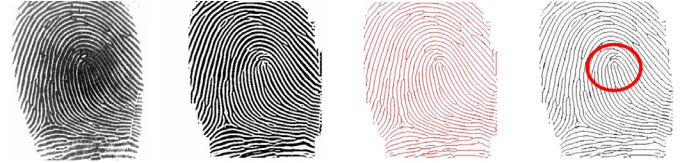
Fig. 13. From the left: original fingerprint, Gabor-filtered fingerprint, thinned fingerprint, ridge reconstructed fingerprint.
