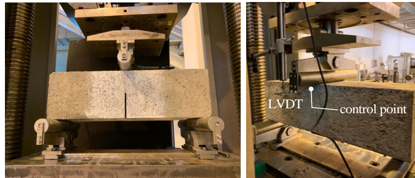
Figure 6. Notched concrete beams tested in three-point bending under displacement-controlled mode.
