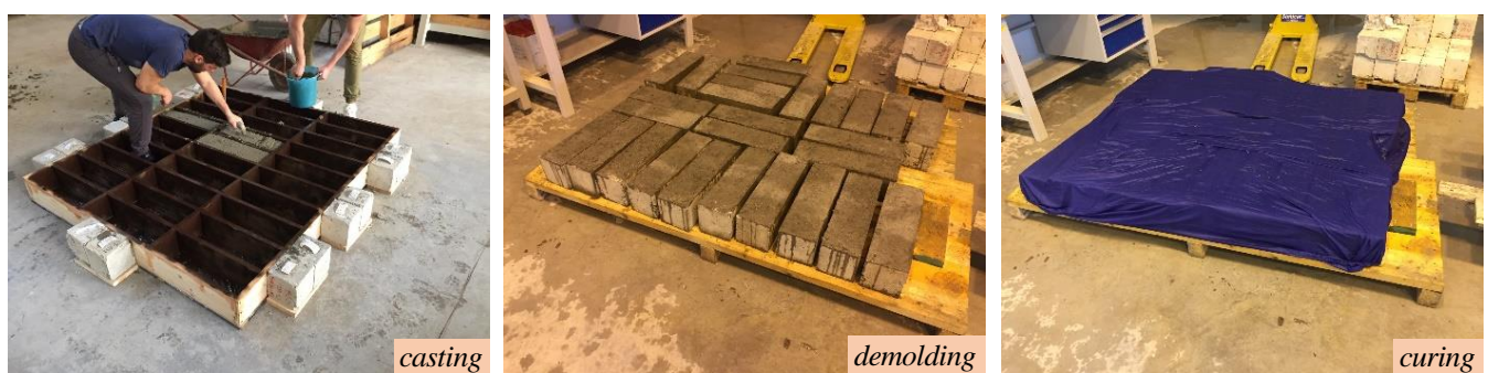
Figure 2. Preparation phases of concrete beams.
