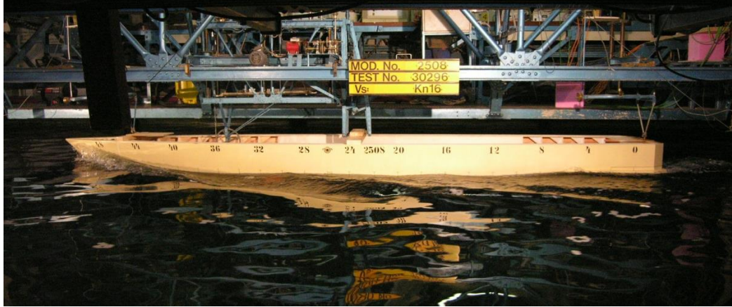
Fig. 3 Model test setup for resistance test [24]
