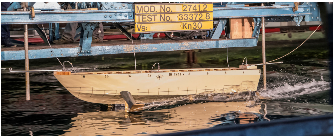
Fig. 8 Seakeeping test of RHS 160 at SVA in Wien
