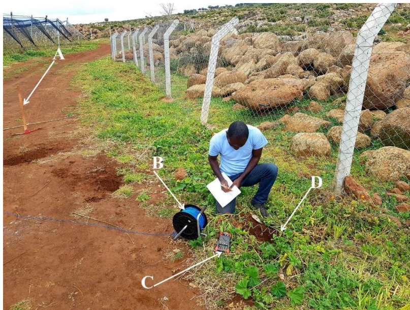
Figure 9. An example of SP measurement station at the ground surface on which a pickaxe (A) is used to dig a shallow hole with 30 cm of depth where one non-polarizing electrode (D) connected to a multimeter (C) and another fixed non-polarizing electrode via an electrical cable (B) is introduced to take SP signal.
