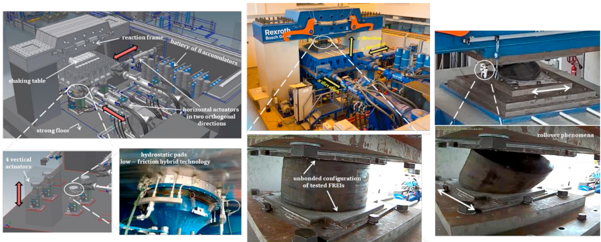
Fig. 2. 3D testing apparatus for full-scale testing of FREIs at the EUROLAB of the University of Messina, Italy.
