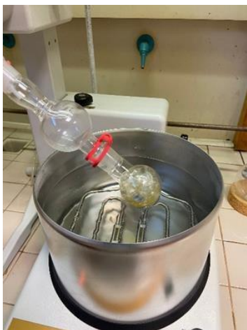
Figure 2.4 Solvent evaporation process with rotary evaporator.
