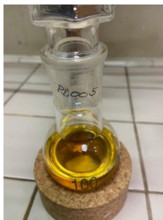
Figure 2.2 Fish oil solid-liquid extraction by stirring at room temperature.
