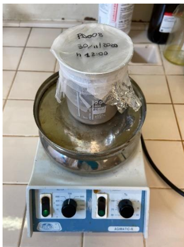
Figure 2.2 Fish oil solid-liquid extraction by stirring at room temperature.
