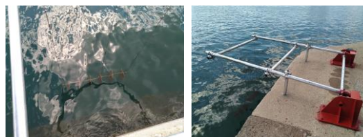
Figure 1 Shipbuilding steel specimens coated with different AF coatings immersed in Palermo's port waters (left). Specimen testing system in immersed position (right).
