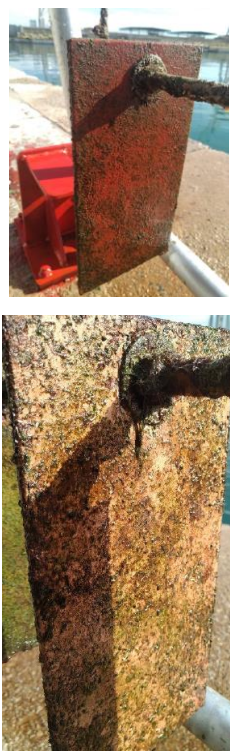
Figure 2 Right side of the shipbuilding steel substrate protected (top) by commercial topcoat and (bottom) by the AquaSun at 5 wt% bismuth tungstate load (THA8-5) after 69 consecutive days in Palermo's harbor waters (13 Sept-22 Nov 2022).
