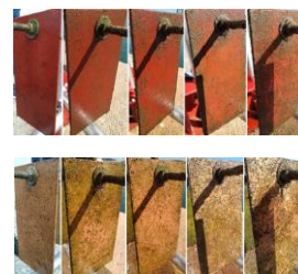
Figure 3 Shipbuilding steel substrate protected by commercial topcoat (top), and by AquaSun doped with 5 wt% bismuth tungstate (bottom) after 14, 28, 42, 56, 69 days immersion in Palermo's port waters (from left to right).
