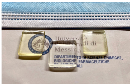
Fig. 3 Photograph of LSCs prepared in this work. In the center, a blank LSC is reported.
