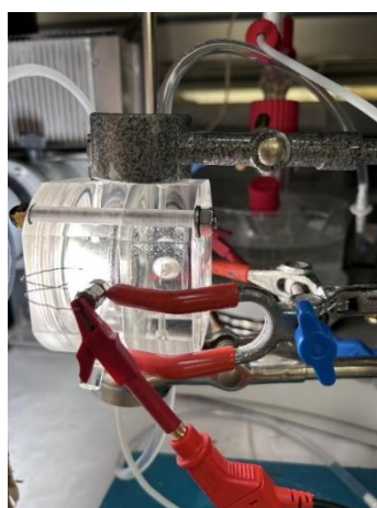
Figure 3.5 Side view of the cell, irradiated by the lamp, during a gas-phase test.
