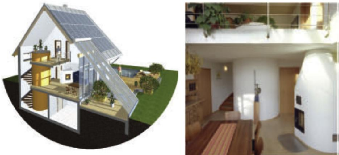
Figure 1.7 Solar heated water tank integrated in the living area of an apartment [78].
