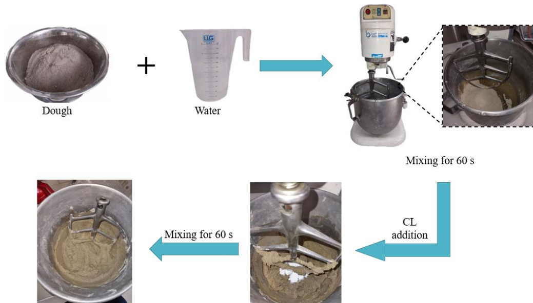
Figure 4.2 Schematic procedure for preparing fresh plaster mortars with CL.
