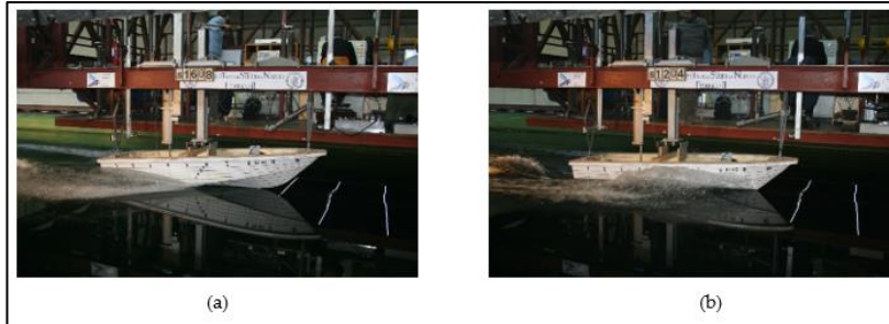
Figure 6. (a) towing tank test with air injection, (b) test without air injection.
