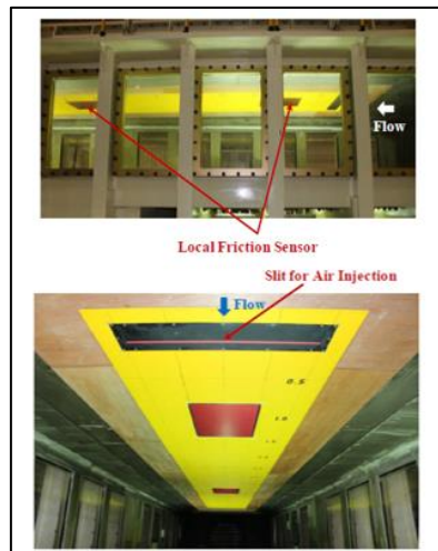
Figure 5. Flat plate in the water tunnel for generation of air layer (reproduced under a CC BY-NC-ND 4.0 DEED license).
