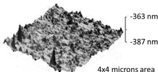
Figure 2: AFM image of a sample calcined at 500 °C and prepared using a 0.1 N concentration of HNO<sub>3</sub> during nanosol. Other parameters as in Figure 1. The RMS value of the film is 1.533 nm.
