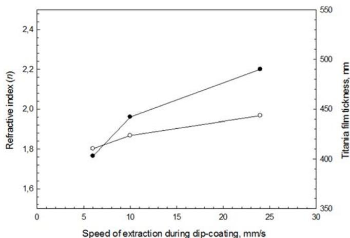
Figure 3: Titania film thickness and refractive index ( $n$ ) for samples calcined at 500 °C, prepared using 0.1 N HNO<sub>3</sub> and 5 coating layers, but variable speed extraction during dip-coating procedure.
