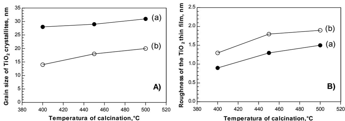
Figure 1: Effect of the calcination temperature on A) grain size of  $\text{TiO}_2$  nanoparticles and B) roughness of the  $\text{TiO}_2$  thin film, for two samples prepared with different concentration of nitric acid during the preparation of the nanosol: 0.1 (a) and 0.5 N (b). Other parameters of preparation: sample prepared by repeating 5 times the dip-coating procedure,  $6 \text{ mm/s}$  as rate used for extracting the sample from nanosol during dip-coating process.
