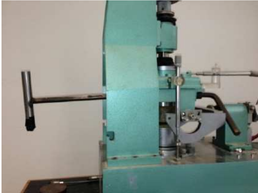
Figure 68 – Detail of the specimen clamping system.
