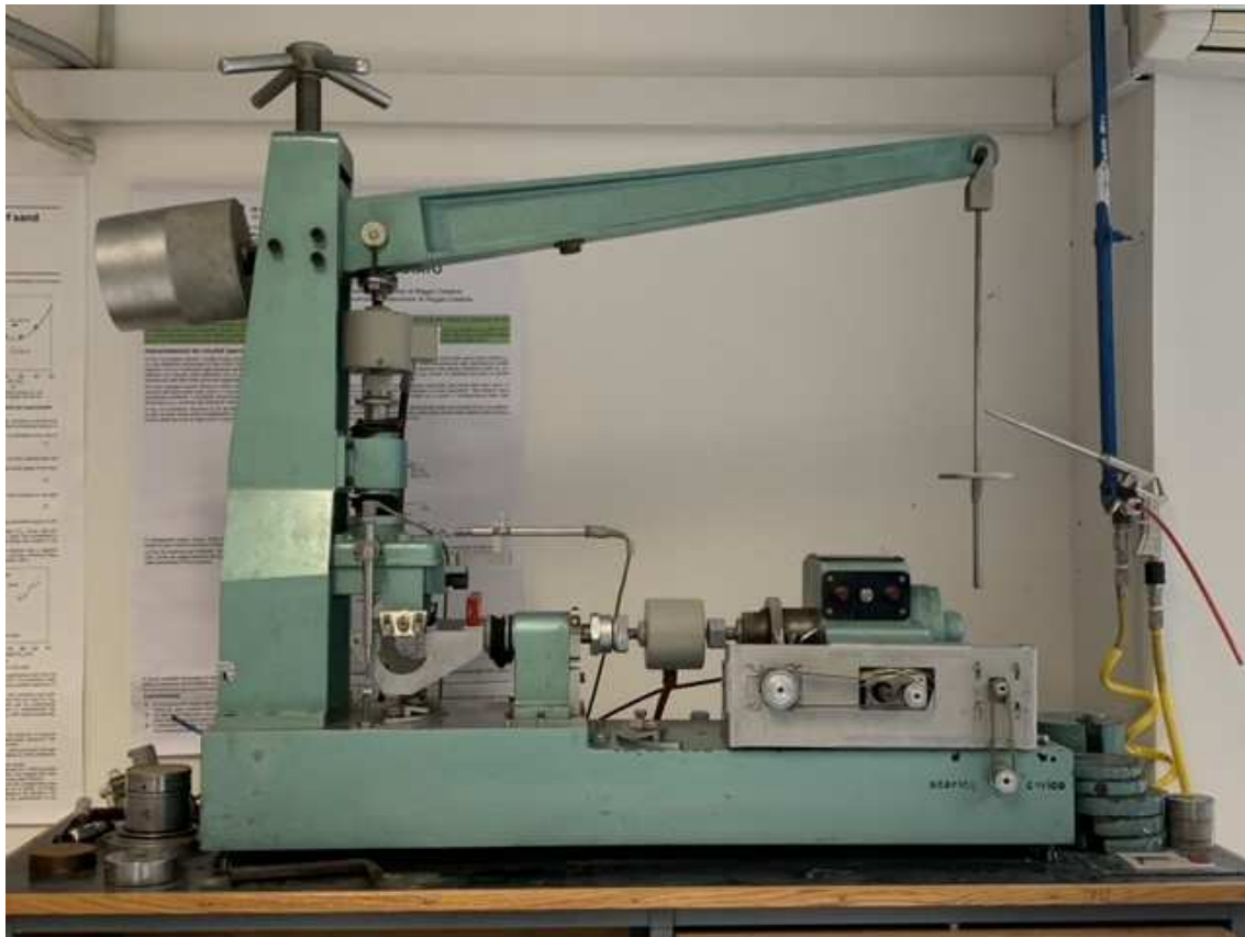
Figure 61 – The modified NGI simple shear apparatus used in the present research.
